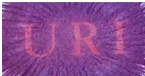
FIGURE 1. A thin film of RR rapidly cooled with a room temperature metal template
