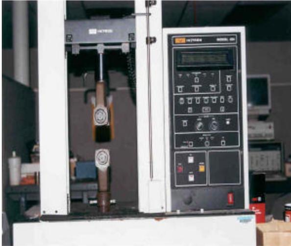
Figure 3. Instron Tensile Tester
