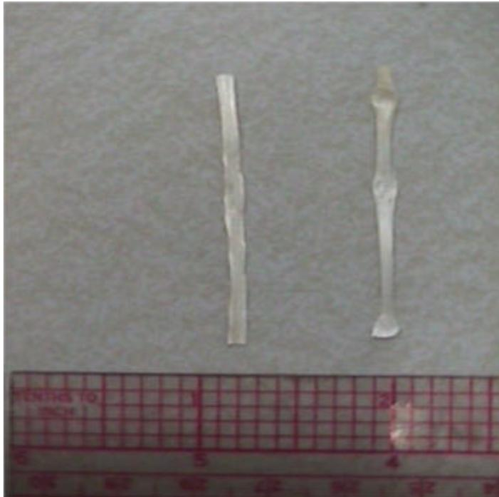
Figure 2. Polypropylene fibers used for reinforcing concrete.
